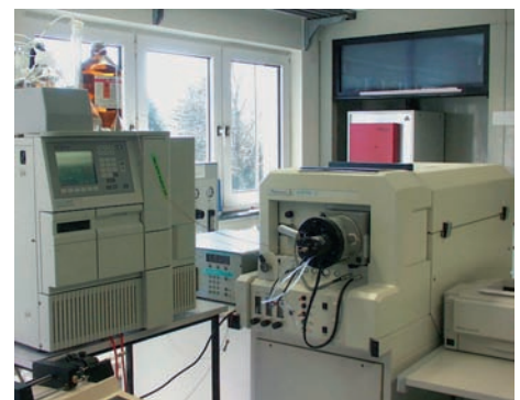
Figure 2: LC/MS/MS unit for the identification of PFTs
